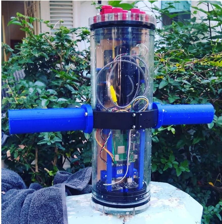
**Figure A2.3:** The MiniEye stereo vision rig, a precursor to the LoCO AUV.
