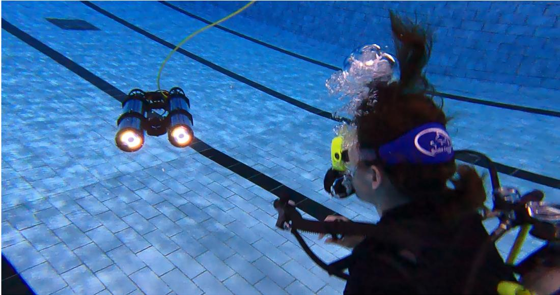
**Figure 3.1:** The LoCO AUV informs a diver that it is ready to follow them, using the active luceme  $L_{FollowYou}$ .
