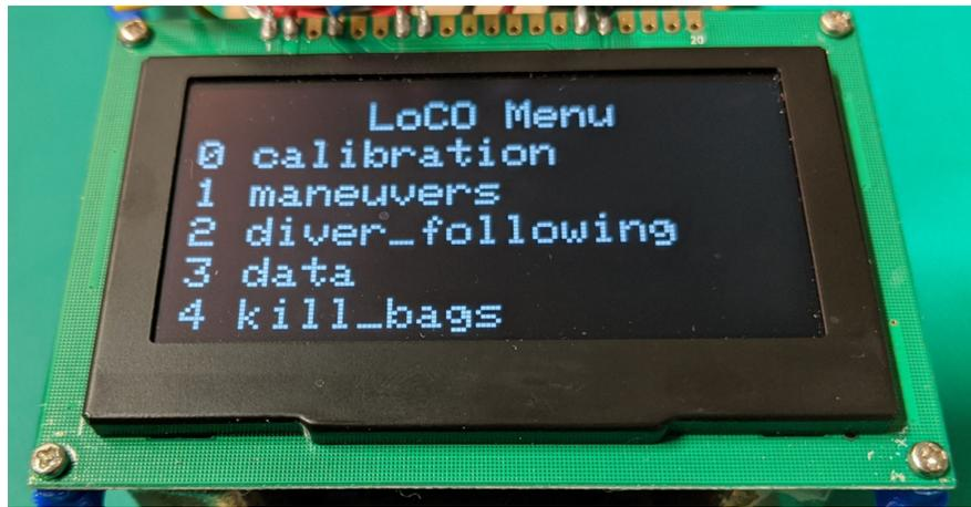
**Figure A2.7:** LoCO's OLED display showing a menu.
