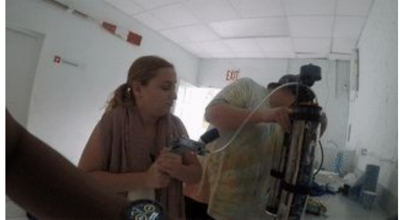
Pumping air out of enclosures to create vacuum seal.
